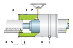
1. Pipe - 2. ProRox® insulation - 3. Cladding - 4. Sheetmetal screw or rivet - 5. Swage - 6. Drainage opening - 7. Straps –  $B \ge 2$ " (50 mm)
