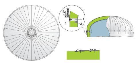
1. Supporting construction - 2. Mounting support
