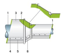
1. Pipe - 2. ProRox® insulation - 3. Cladding - 4. Sheet-metal screw or rivet - 5. Swage - 6. Reducer
