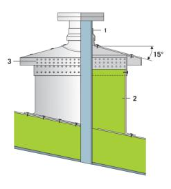
1. Sealing tape - 2. ProRox® insulation - 3. Perforated sheet (ventilation)
