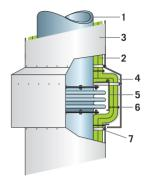
Pipe - 2. ProRox<sup>®</sup> insulation - 3. Cladding Aluminum foil - 5. Cover sheet - 6. Wrap (mat) pin with clip - 7. Spacer
