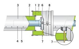
1. Pipe - 2. ProRox® insulation - 3. Cladding - 4. Sheetmetal screw or rivet - 5. Swage - 6. Flange band - 7. Leak detection fitting - 8. Clamps
