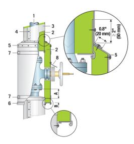
1. Pipe - 2. ProRox® insulation - 3. Cladding - 4. Sheetmetal screw or rivet - 5. Rain deflector - 6. Lock washer - 7. Straps - 8. Rain deflector -  $B \ge 2$ " (50 mm) - A = bolt length + 1.2" (30 mm)
