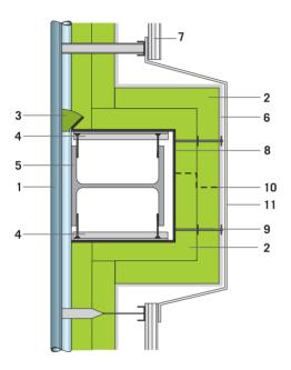
1. Boiler wall - 2. ProRox® insulation - 3. Fill up with loose fill stone wool (mineral wool) - 4. Support construction - 5. Buckstay exposed to heat - 6. Aluminum foil if required - 7. Cladding/Preformed sheet - 8. Internal buckstay cover, made from black sheet - 9. Mat pins with clips - 10. Aluminum foil barrier - 11. Flat sheet cladding
