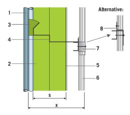
1. Boiler wall - 2. ProRox® insulation - 3. Fill with loose rock wool - 4. Convection barrier sheet - 5. Aluminum foil if required - 6. Metal cladding - 7. MF profile filling - 8. Z-profile separating sheet
