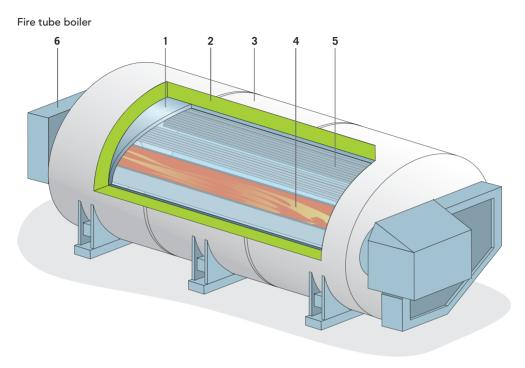
1. Boiler casing - 2. ProRox® insulation - 3. Cladding - 4. Flame tube - 5. Fire tube - 6. Reversing chamber
