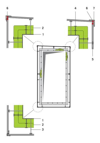
1. Duct wall - 2. ProRox® insulation - 3. Support construction and spacer - 4. Welding pins/clips - 5. Metal cladding: corrugated sheet - 6. Extension (trapezoid) - 7. Z-shaped spacer
