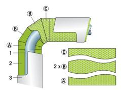
1. Pipe - 2. ProRox® insulation - 3. Cladding - A to C: Elbow segments of wraps (mats)
