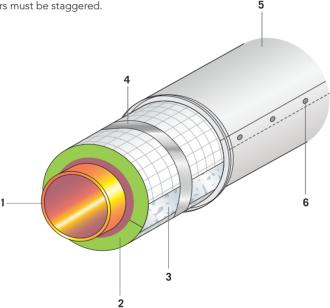
1. Pipe - 2. Insulation: ProRox $^{\circ}$  MA 960 $^{\text{NA}}$  - 3. Self-adhesive aluminum tape - 4. Steel bands - 5. Sheet cladding - 6. Sheet-metal screw or rivet
