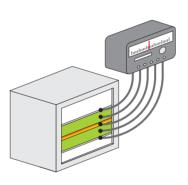
The core components of the apparatus usually consist of two cold-surface units and a guarded hot-surface unit. The insulation material to be measured is sandwiched between these units. The thermal conductivity is calculated at the mean temperature between the hot and the cold side and expressed at the hot face temperature.
