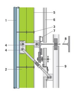
1. Boiler wall - ProRox® insulation - 3. Mat pins with clips - 4. Buckstay deflectors - 5. Aluminum foil if required - 6. Metal cladding/profiled sheet - 7. Substructure - 8. Cold buckstay - 9. Boiler handle
