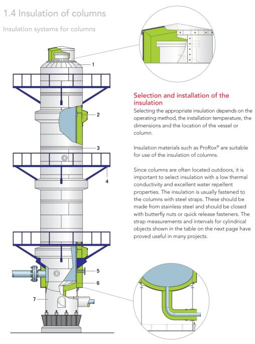
1. Column head - 2. Reinforcement ring - 3. Expansion joint - 4. Working platform - 5. Identification board -
