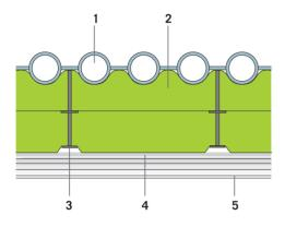
Tube wall - 2. ProRox® insulation – 3. spring plates Aluminum foil if required - 5. Cladding (e.g. profiled sheet)
