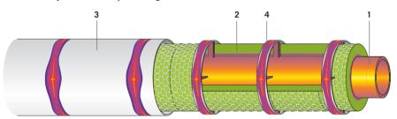
1. Pipe - 2. Insulation: ProRox® Wired Mats - 3. Cladding - 4. Spacer ring
