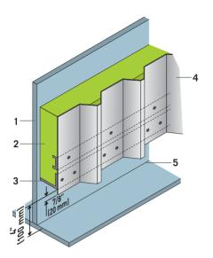
1. Tank wall - 2. ProRox<sup>®</sup> insulation - 3. Support ring - 4. Cladding - 5. Welded seam
