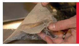
Reinforced polyester wrap (mat) positioned between two sheets of film.
