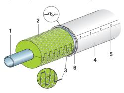
1. Pipe - 2. Insulation: ProRox® Wired Mats - 3. Stitching of the joint edge with binding wire - 4. Sheet cladding - 5. Sheet-metal screw or riveted bolt - 6. Spacer ring
