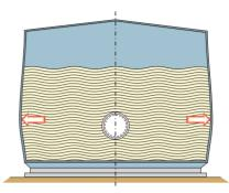
the tank diameter. Example: The diameter of a storage tank - Ø 65 ft (20 m), Avg T 430 °F (220 °C) - will increase approx. 2 1/2" (60 mm). This consequently increases the tank circumference by approx. 7" (180 mm). To avoid stress/tension on the insulation protection (aluminum sheeting) selecting flexible ProRox® insulation board (slab) or wrap (mat) is important. For high temperatures, anticipate further expansion by fitting profiled sheeting.
