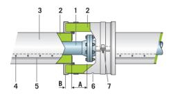
1. Pipe - 2. ProRox® insulation - 3. Cladding - 4. Sheetmetal screw or rivet - 5. Swage - 6. Drainage opening - 7. Straps –  $B \ge 2$ " (50 mm) -  $A = Bolt \ length + 1.2$ " (30 mm)
