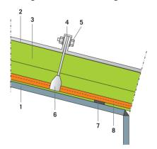
1. Tank roof - 2. Cladding - 3. ProRox® pressure resistant insulation - 4. Aluminum finishing strip - 5. Bolts and rivets (stainless steel) - 6. Strip (stainless steel) - 7. Weld - 8. Welded steel bar
