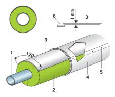
1. Pipe - 2. Insulation: ProRox® PS 980<sup>NA</sup> Pipe Sections - 3. Reinforcement sheet (may not be required) - 4. Cladding - 5. Sheet-metal screw or rivet - 6. Joggle
