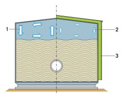
1. No insulation: strong convection - 2. Insulation: reduced convection - 3. ProRox® insulation
