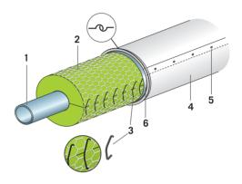
1. Pipe - 2. Insulation: ProRox® Wired Mat- 3. Joint edge closed with mat hooks - 4. Sheet-metal cladding - 5. Sheet-metal screw or riveted bolt - 6. Spacer ring
