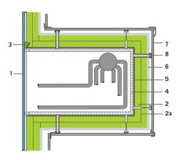
1. Boiler wall - 2. ProRox® insulation - 3. Fill up with loose fill stone wool (mineral wool) - 4. Support construction - 5. Dead space sheeting - 6. Aluminum foil if required - 7. Metal cladding/Preformed sheets - 8. Support construction and spacer
