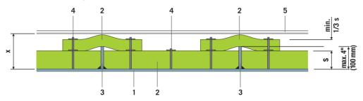
1. Duct wall - 2. ProRox® insulation - 3. Reinforcing ribs - 4. Welding pins with clips - 5. Metal cladding
