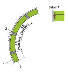
1. Tank wall - 2. Spacer - 3. ProRox® insulation
