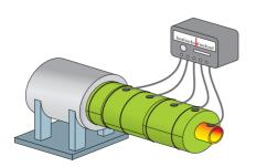
The core consists of a hot pipe with a length of 10 feet (3m). The thermal conductivity is calculated at the mean temperature between the hot and cold side and expressed at the mean temperature. The main difference is that the hot pipe apparatus test method includes the seams within the insulation. This explains why the measured values will be higher than the guarded hot plate apparatus test.
