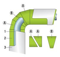
Pipe - 2. Insulation: ProRox® Pipe Sections Cladding - A and B = Segmented pipe sections
