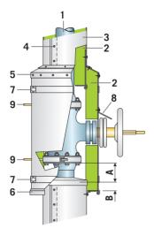
1. Pipe - 2. ProRox® insulation - 3. Cladding - 4. Sheetmetal screw or rivet - 5. Collar - 6. Collar - 7. Clamps - 8. Rain deflector - 9. Leak detection fitting -  $B \ge 2$ " (50 mm) - A = bolt length + 1.2" (30 mm)
