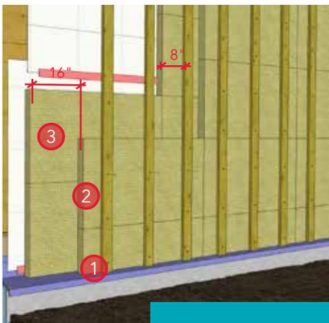
An alternative installation approach is to use one or two fasteners with washers to pin the insulation boards in place before the strapping is installed.
