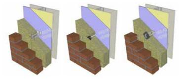
Examples of alternate masonry ties installed through ROCKWOOL CAVITYROCK  $^{\circ}$  insulation.
