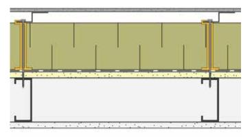
Uninsulated 3 5/8" steel stud wall with exterior insulation and cladding attachment system.
