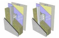
Additional examples of thermally isolated galvanized steel clips where low-conductivity pads are used to reduce the heat flow through each clip. Note that the best performance arises when the continuous girts attached to the clips are entirely outboard of the insulation and do not cut through it.
