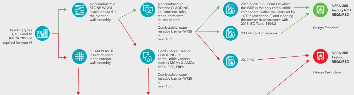
While foam plastic insulation triggers the need for NFPA 285 testing, noncombustible ROCKWOOL insulation does not, and it is often used in conjunction with combustible claddings and/or water-resistive barriers to help achieve successful NFPA 285 test results.
